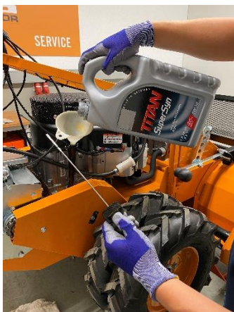
Figure 4: For 4-stroke engines the oil level must be checked and, if necessary, missing oil topped up.
