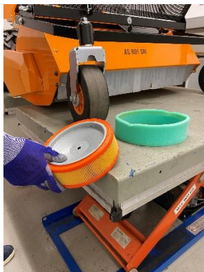
Figure 3: Gently tap the air filter to remove dry dust, plant seeds and foreign matter.
