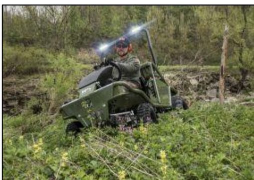
Photo 3: The special edition has two additional 18-watt LED headlights and a transport box
