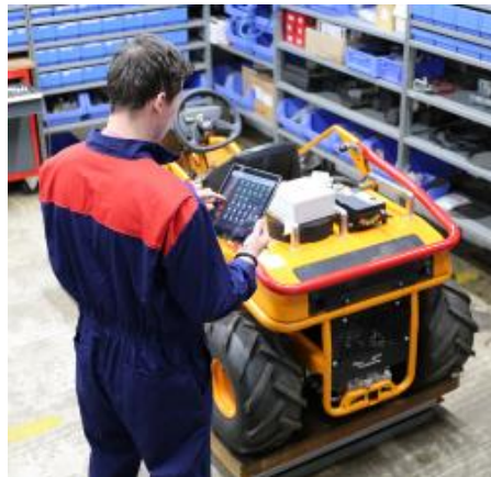
Photo 2: The AS SherLog1.0 diagnostic device makes it possible for the servicing dealer to carry out a test within a few minutes in the workshop or on site
