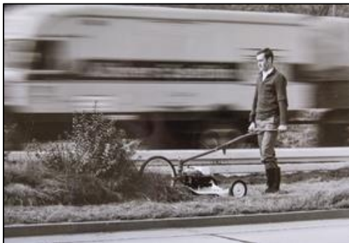
Photo 1: Alfred Schefenacker developed the first Allmäher for use on steep slopes, in vineyards and for rarely mown meadow orchards
