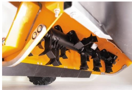
Photo 4: AS 1040 Yak 4WD’s flail mowing unit
